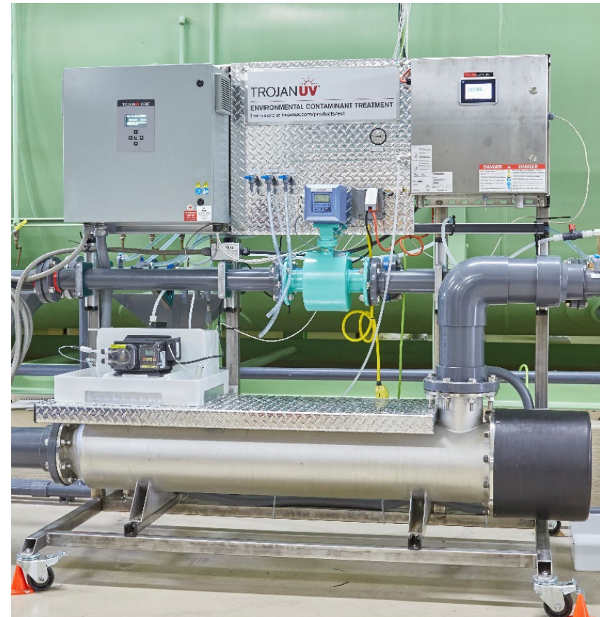
Trojan UVPhox Pilot System (low pressure UV lamps)
